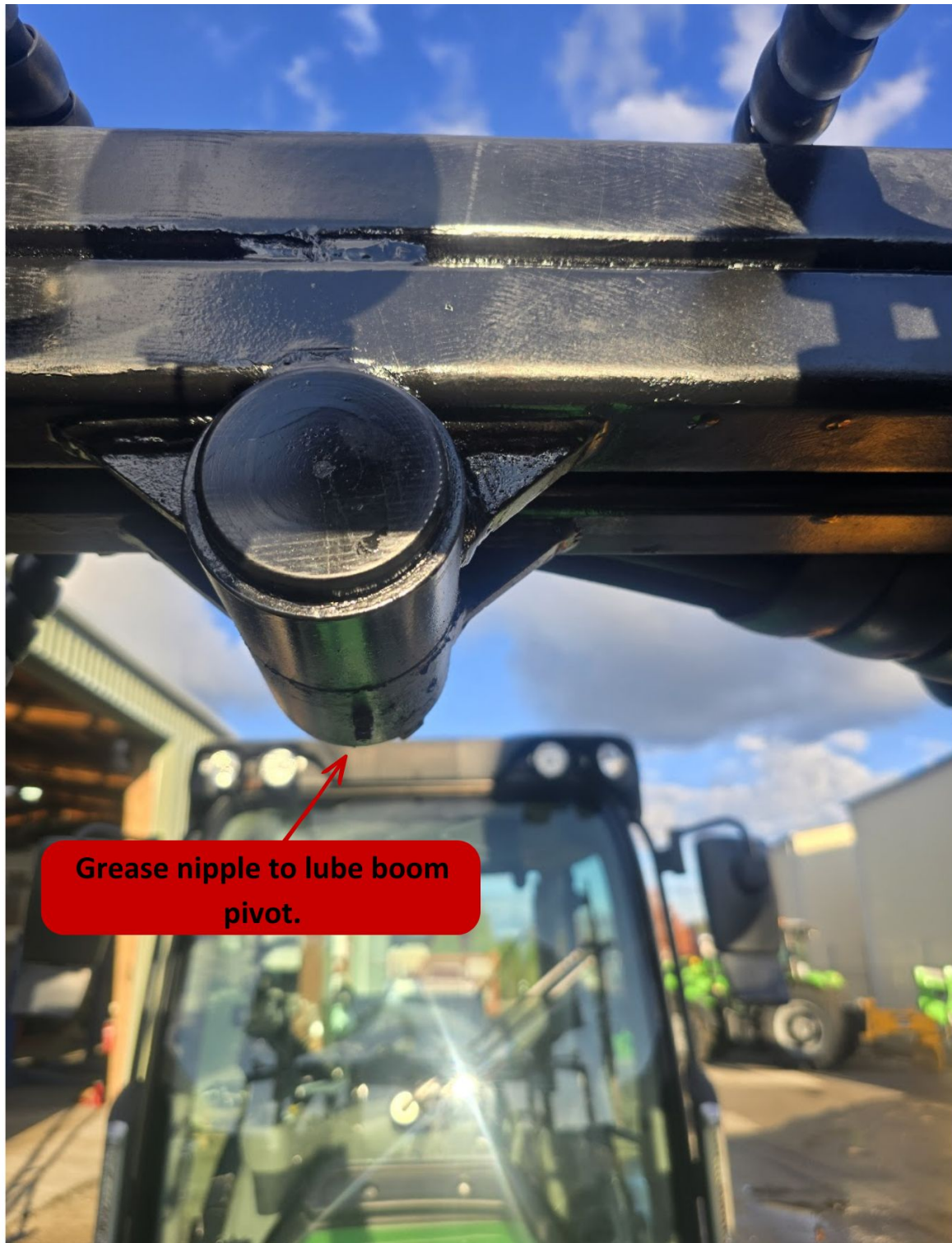
Grease boom pivot pin
